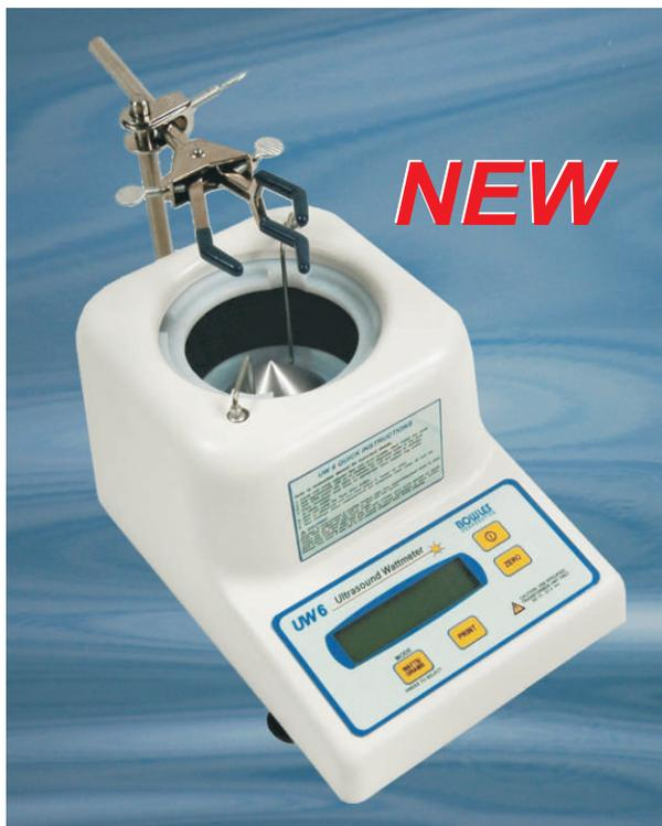
The UW 6 Digital Ultrasound Wattmeter is designed to provide an accurate means of verifying and calibrating the output of therapeutic ultrasound devices. The meter measures the ultrasound power output utilizing a state of the art microprocessor and strain gauge bridge transducer to provide quick, reliable readings.
