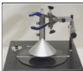
The cone target and transducer positioner. (Tank not shown.)
